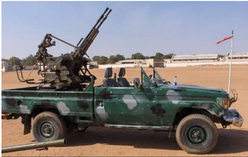
Figure 1 Twin-barrel 14.5-mm machine gun (on Government of the Sudan vehicle for display only)
